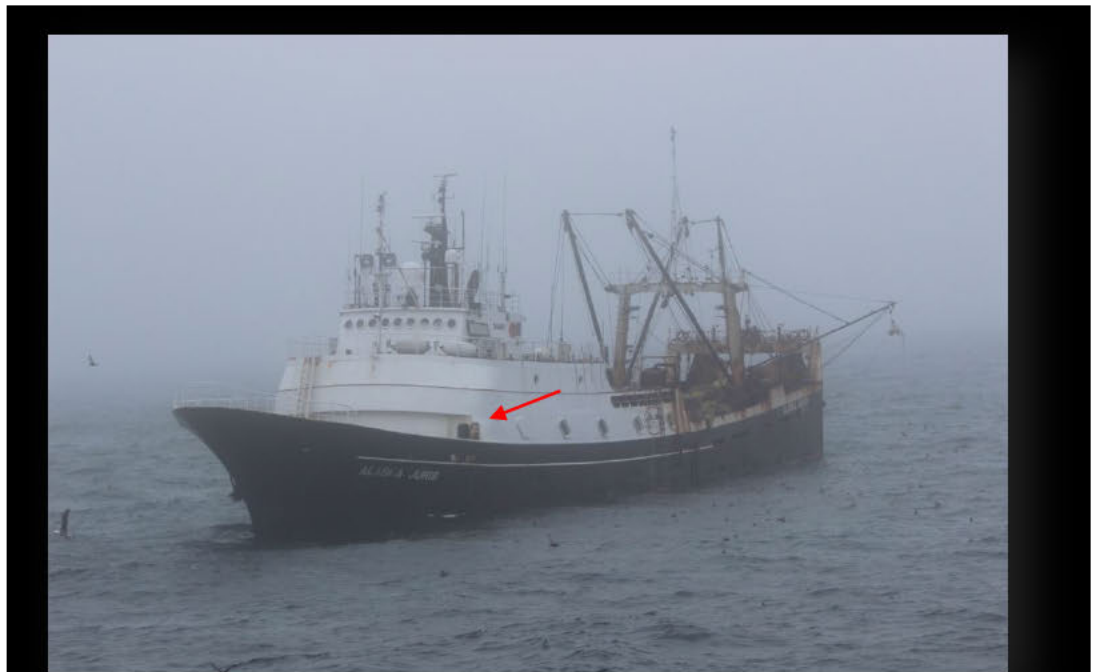
Figure 4.L. Photo of the ALASKA JURIS with has a red arrow pointing to a watertight door that was routinely left open by crew to provide ventilation to the living quarters in the house. Photo was taken from the SEAFISHER approximately 7 hours after the abandonment on July 26, 2016.
