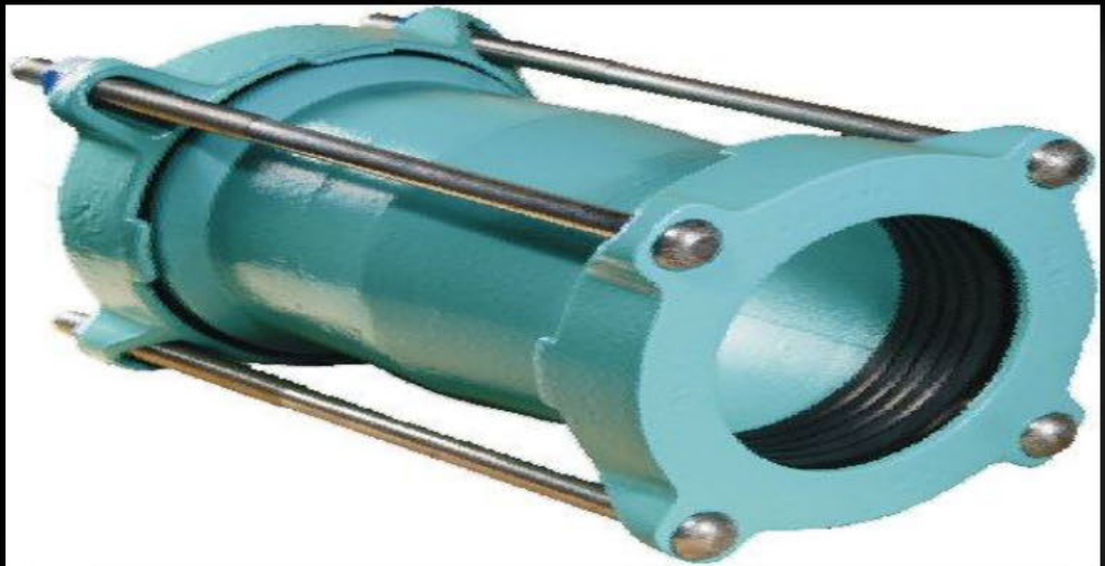
Figure 4.O. This is an example of what a mechanical coupling on the ALASKA JURIS looked like. Note: Mechanical couplings are used to join pieces of pipe in lieu of welding or bolting flanged joints. Once installed on a pipe, the bolts on the mechanical coupling are tightened and the gasket material on either end of the coupling is compressed onto the pipe to create a seal. They are sometimes used in lieu of repairing wasted pipe or to join misaligned pipe.
