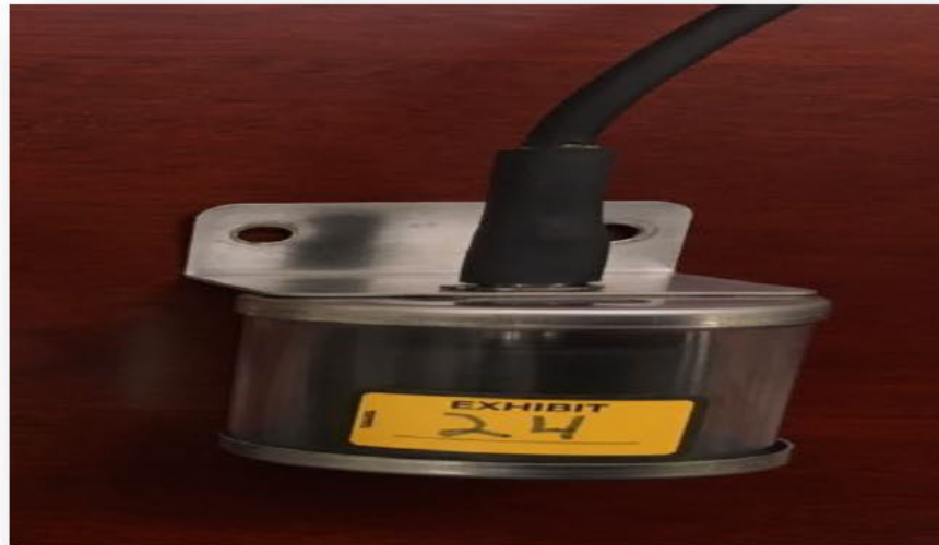
Figure 4.M. Photo of the type of high bilge alarm float switches installed on the ALASKA JURIS.
